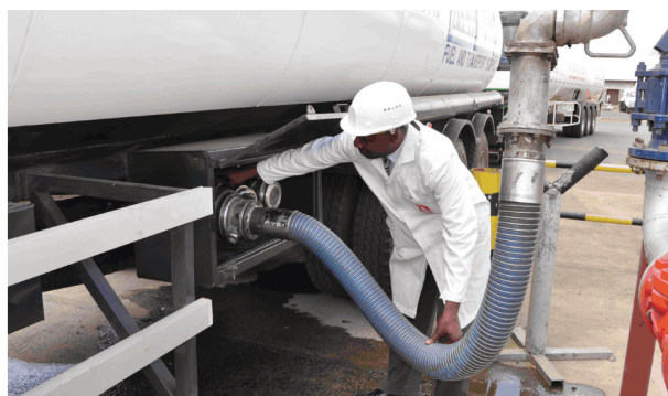
Bottom loading of petroleum products.
